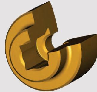
**Cornering Inserts** – Machine Squares, Hexagons, and Octagons with Inserts designed with two cutting edges intersecting at the appropriate angle 90, 120 or 135 degrees. Cut the corner, rotate the spindle (C axis) as required for the next cut (re-run of the subroutine) and repeat to completion. The same cornering Inserts may be used to generate a range of sizes of the given shape by simply increasing or decreasing the tool offset.
